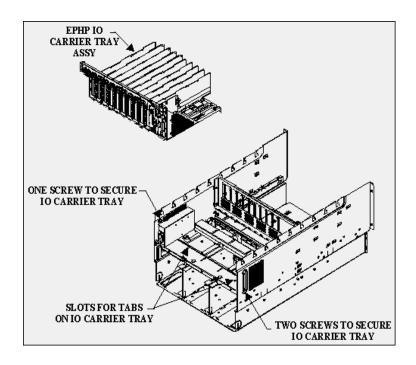
Figure 2-13: Installing the I/O Carrier Tray
